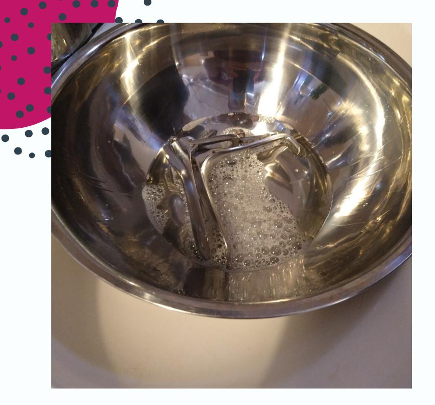
Step 6: Place the instrument into 10% solution chlorine, let it sit for 20 seconds.
